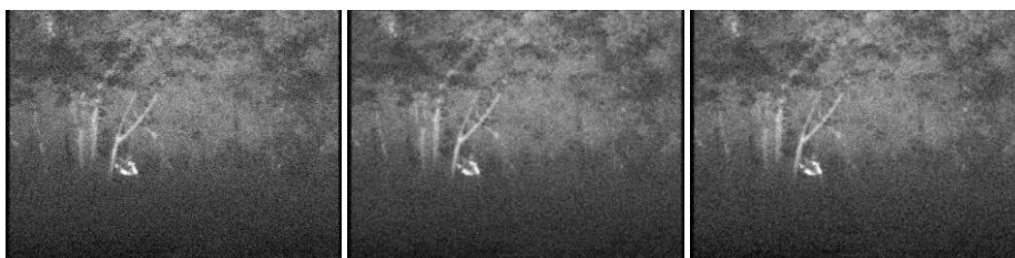
(g)Add gaussian noise figure (h) Gaussian 3x3 average filter (i) Gaussian 3x3 median filter
