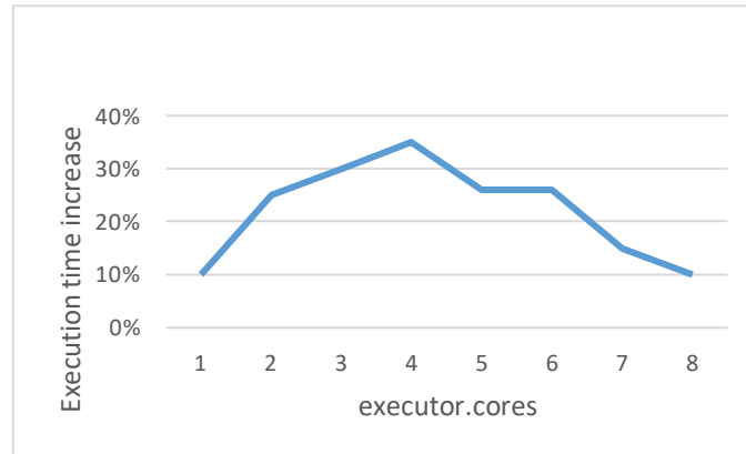
Fig.6 The amount of execution time increase of TeraSort varies with the number of CPUs.
