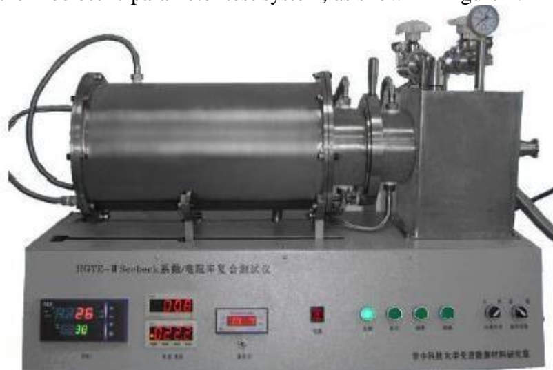
Fig. 4 hgte-ii thermoelectric parameter test system
