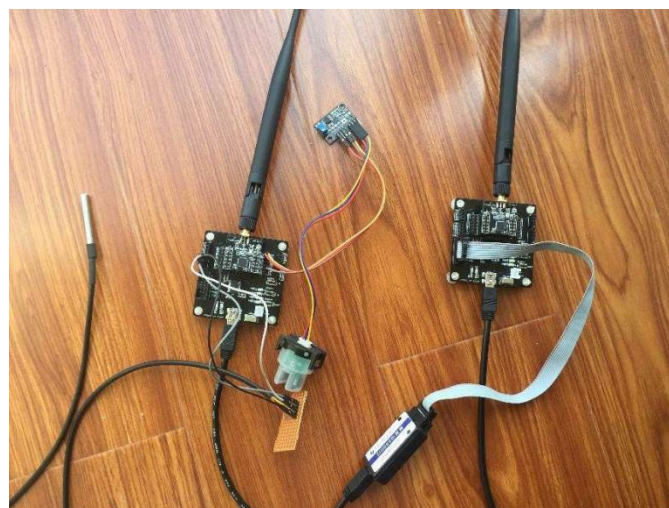
Figure 2-23 Overall physical connection diagram of the system
